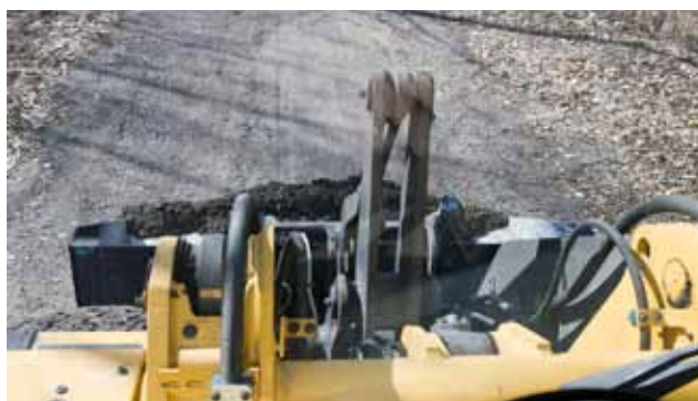
The grading bucket has a long bottom, giving the driver a good view and complete control of the work.
